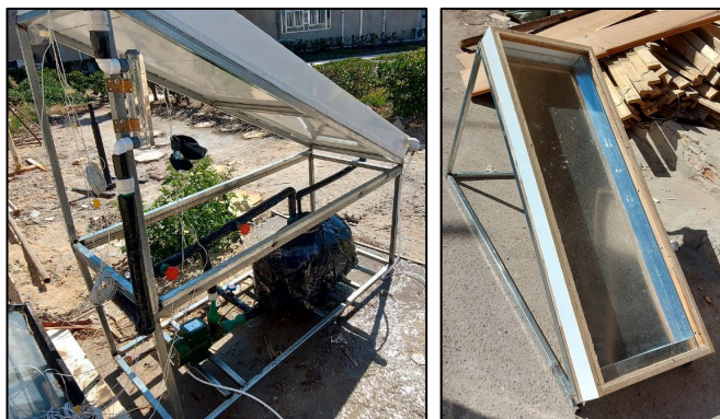
Fig. 6 Inclined base structure.
