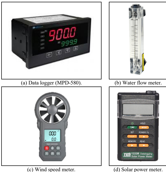
Fig. 8 Measuring equipment used in this study.
